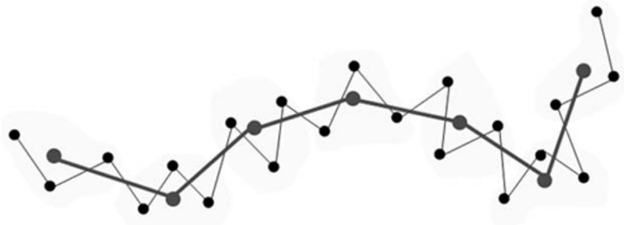
Figure 1. Selection of coarse-level variables for a polymer. Each pseudoparticle at the next-coarser level (large dots) is placed at the geometric center of three fine-level atoms (small dots).
