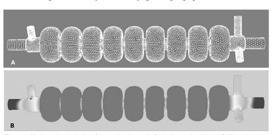
**Figure 1.** Mesh used in the design of the accelerating cavity for the International Linear Collider (A) and the resulting computed electric field distribution of the accelerating mode (B). Courtesy of the Advanced Computations Department, SLAC.
