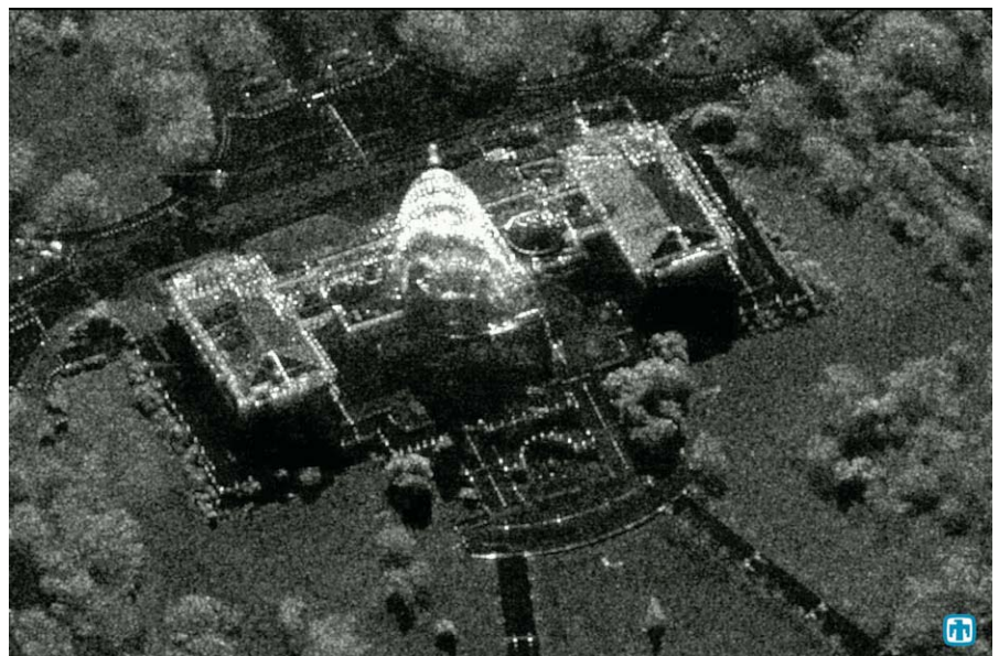
Figure 2. SAR image of the U.S. Capitol. The dome is distorted, an effect that arises from the assumption that scatterers lie on a flat surface. Interferometric SAR is a two-antenna technique that can be used to find the surface shape. Could the surface be found from single-antenna data? Image from Sandia National Laboratories.
