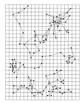
**Figure 1.** Brownian motion. The positions of three granules of mastic were recorded every 30 seconds by Jean Perrin. Each 30-second position was connected by a straight line, which reveals the zig-zagging path of the granule. From Einstein 1905.
