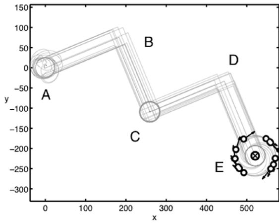
**Figure 4.** Twelve point particles starting in random positions near  $(0,0)$  first congregate in a circle, then head off in an east-northeast direction (A), shift to the southeast (B), pause in a circular formation before repeating the zigzag (C and D), and end by enlarging the circle (E). From Rodolphe Sepulchre, Derek Paley, and Naomi Ehrich Leonard, "Stabilization of Planar Collective Motion, Part I: All-to-All Communication," 2005.
