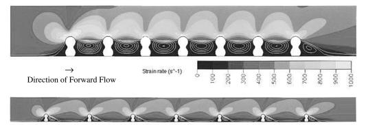
**Figure 3.** Strut spacing has been implicated in the stagnation or eddies in blood flow seen in many patients with stents. Simulations by James Moore and colleagues show grayscale-encoded strain rates for two strut spacings in a Wallstent; the eddies and pooling seen with closely spaced struts (above) are replaced by flow reattachment with wider spacing (below). From Annals of Biomedical Engineering, Vol. 30, 2002, reprinted with the permission of the Biomedical Engineering Society.
