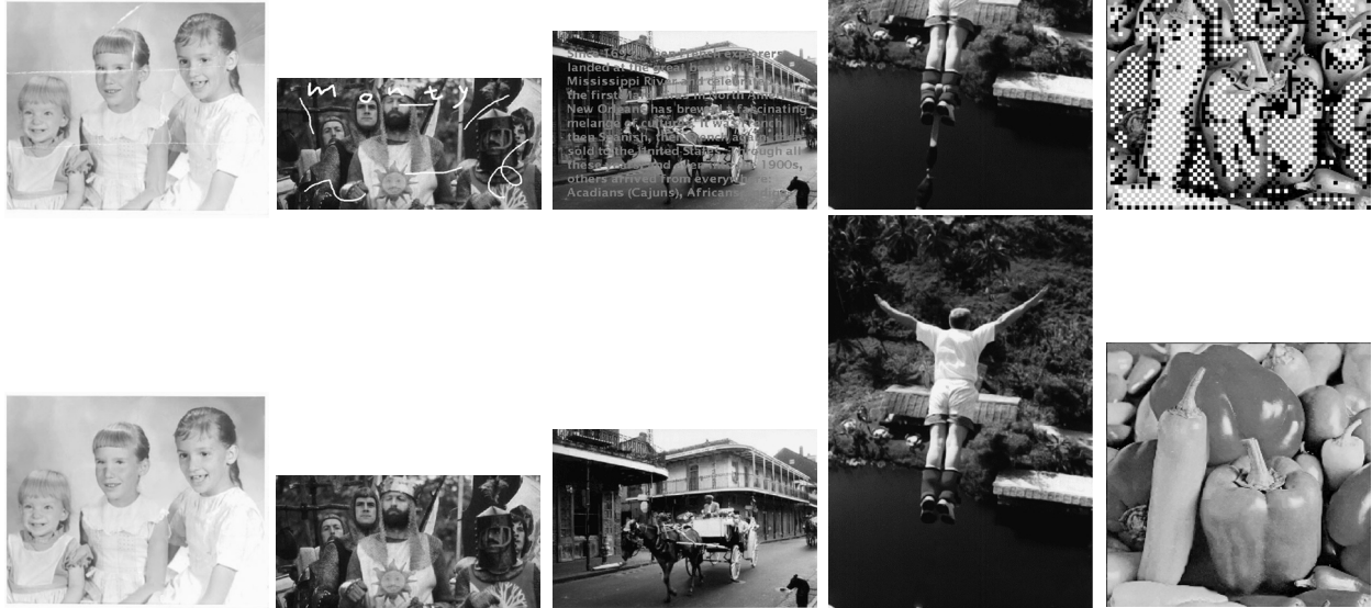
Figure 2. Original images (top row) after inpainting (bottom row) for, respectively, the restoration of damaged photographs, restoration of scratched film, text removal, object removal for special effects, and block reconstruction in wireless transmission.
