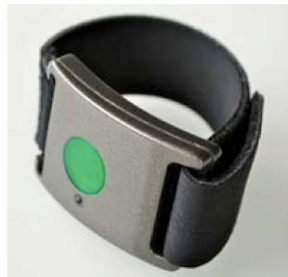
Figure 1. Affective Q™ Sensor is a wrist-worn commercial sensor that monitors: 1) EDA, 2) skin temperature and 3) 3-axis accelerometer.
