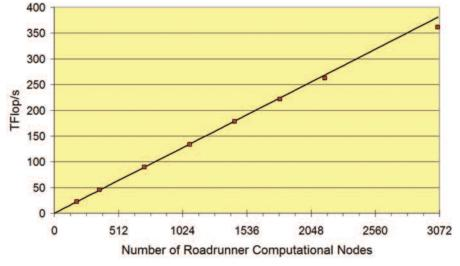
**Figure 2**. Near-ideal scaling and sustained double-precision performance of 361 teraflop/s have already been achieved for the molecular dynamics code SPaSM on Roadrunner.
