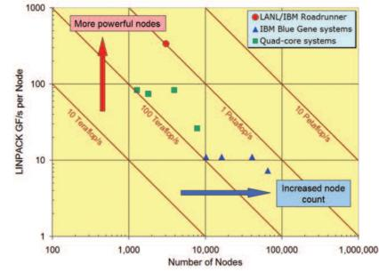
**Figure 1**. With fewer, more powerful hybrid nodes, Roadrunner represents a different path to petascale computing.
