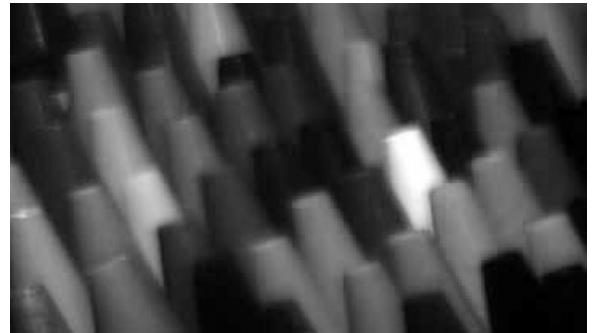
Crayons seen through a cubic phase plate, unprocessed and uniformly out of focus.
