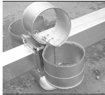
Figure 3. Inertial effects on shard curls. Left, at speeds of 30 to 40 km/h, the shards come off the mandrel and form a relatively tight curl. Right, in full-scale crash tests at higher speeds (about 100 km/h), inertial effects cause a much looser curl on the shards.
