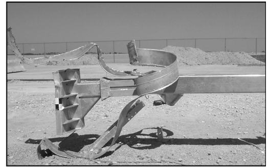
Figure 3. Inertial effects on shard curls. Left, at speeds of 30 to 40 km/h, the shards come off the mandrel and form a relatively tight curl. Right, in full-scale crash tests at higher speeds (about 100 km/h), inertial effects cause a much looser curl on the shards.
